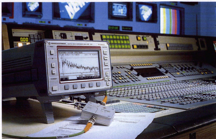
FIG 1 Digital Video Component Analyzer VCA, specialist for in-depth analysis of digital video signals Photo 42 246/1
