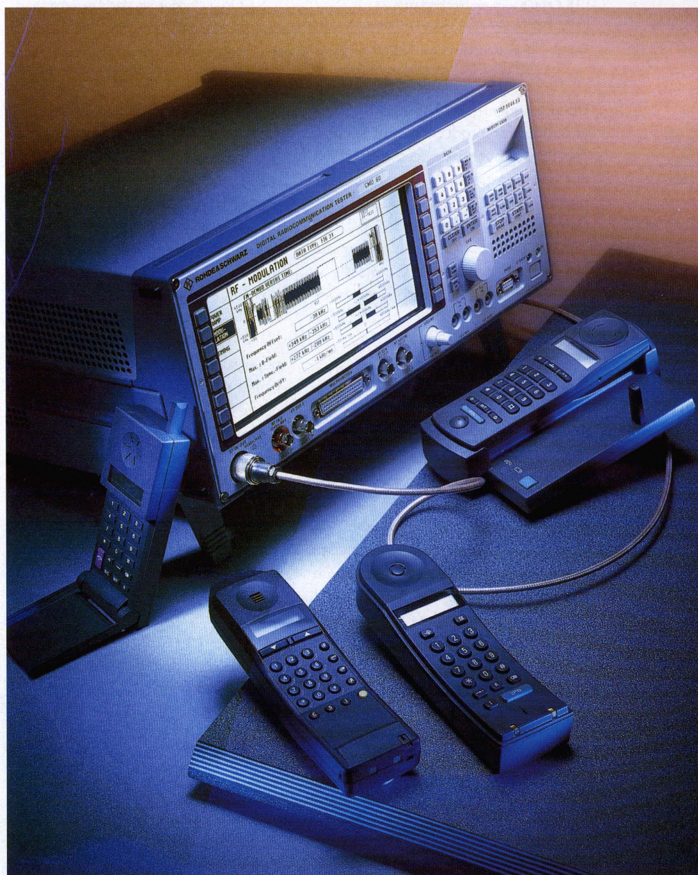
FIG 1 Rapid, precise and complete measurements by Digital Radiocommunication Tester CMD60 are prerequisites for cost-effective volume production of cordless telephones in line with DECT standard. Photo 42 204
