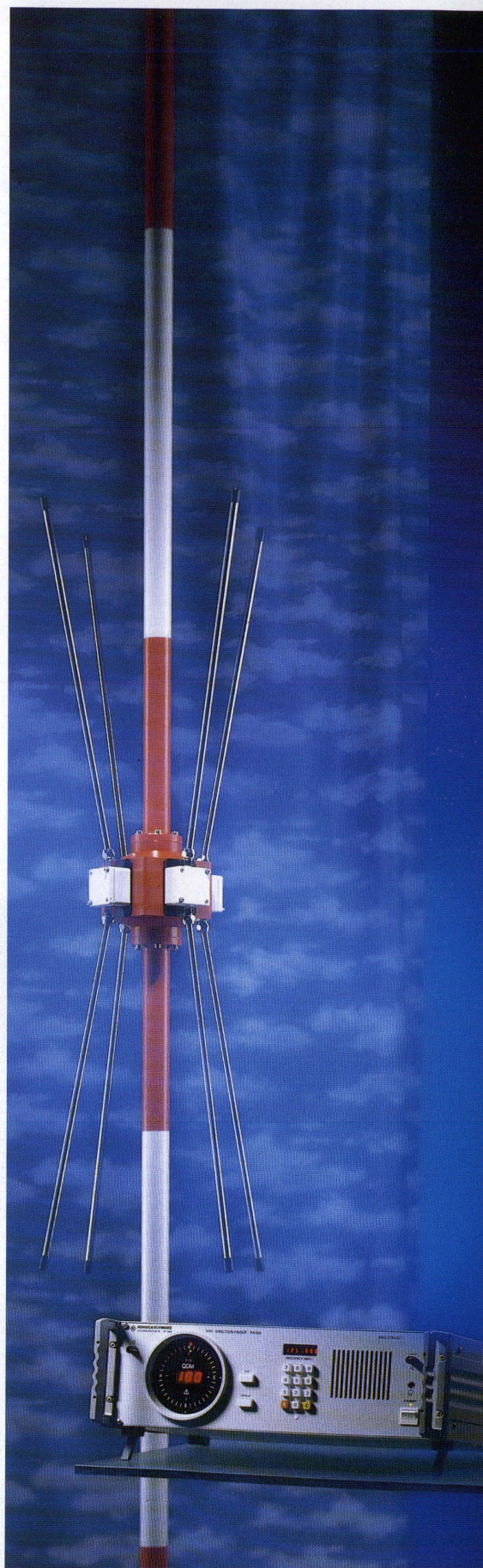
FIG 1 VHF Direction Finder PA030 with compact, sturdy antenna and detached bearing display for wide field of application at airports Photo 42 216/2
